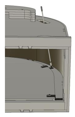
Use [the supplied] <sup>3</sup>/<sub>8</sub>" long hex head screws to anchor each bracket to the rim.
